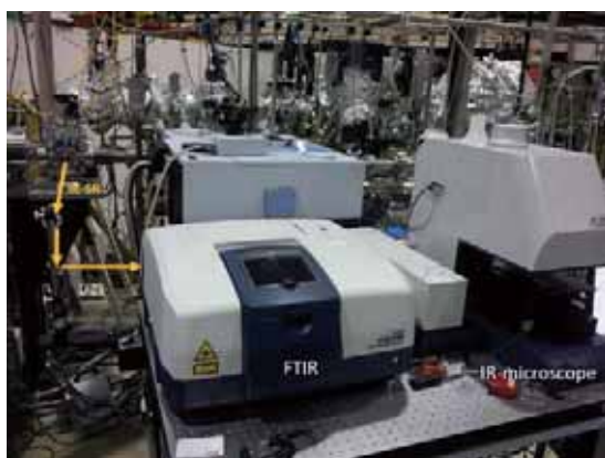
Fig. 1. Layout of the IR microspectroscopy (IR-MS) apparatus installed at BL6B. The infrared synchrotron radiation (IR-SR) is introduced to the IR-MS by two plane mirrors through the atmosphere.
